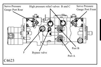
NOTE: Internal charge pump model shown
