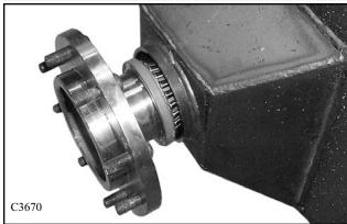
11 Place 2 seal installation tools, Thomas P/N 958674, equally spaced around the axle flange, behind the seal. (fig. C3671). This special tool must be used to properly locate the seal into the final drive housing.
