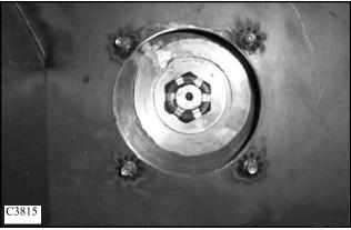
14 Tighten the castle nut and guide the axle into the final drive housing as straight as possible to prevent damaging the seal. Tap the axle flange with a hammer if necessary to assist the installation.
