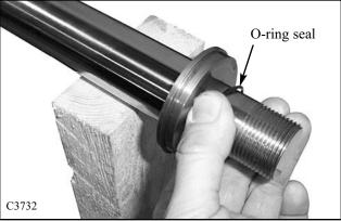
9 Remove the gland nut assembly from the cylinder rod. (fig. C3733)
