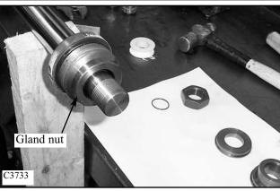
10 Remove and discard the wiper seal, rod seal and oring seals and teflon back up washer, (if used), from the gland nut assembly. (fig. C3734) NOTE: Some seal designs may vary from illustration
