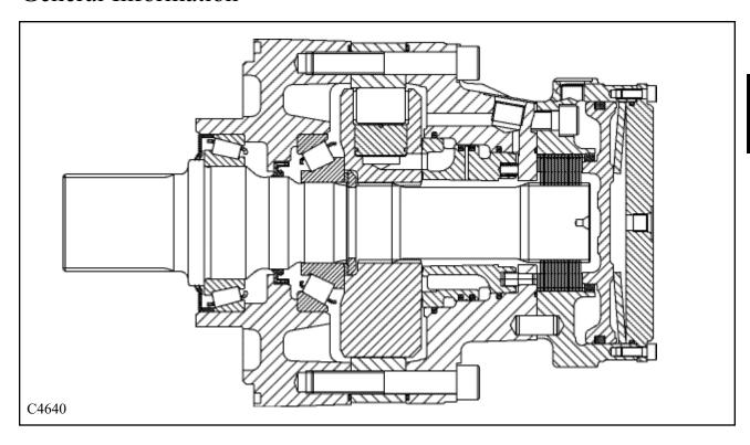
The basic radial piston design uses a combination of mechanical and hydraulic principles that are utilized in the high torque, low speed motors.
