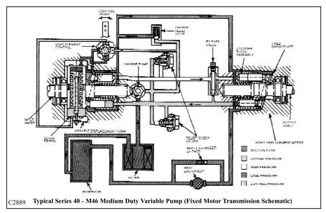
The M46 Medium Displacement pumps can be applied separately or combined in a system to transfer and control power. When combined in such a system, these units provide an infinitely variable speed range between zero and maximum, in both forward and reverse modes of operation.
