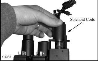
3 Remove the screws retaining the solenoid assembly to the control valve. (fig. C4239). Upon assembly tighten the screws to 5 ft lbs (7 Nm).
